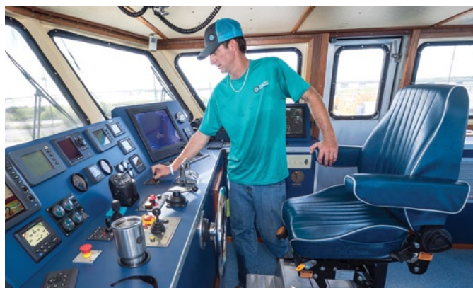
Capt. Kyle Plaisance turns on J.L. O'Brien's bridge electronics. In addition to the latest navigation equipment, the 95-foot OSRV has an infrared system for detecting oil spills at night.
